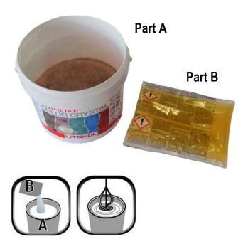
Mix using an electric drill with the paddle at low speed until achieving a smooth mixture without lumps. When the 2 components are properly mixed you will notice a homogeneous, uniform paste without color variation. Scrape the sides and bottom of the bucket with a spatula or trowel to ensure complete and proper mixing. It is never advisable to mix by hand.
