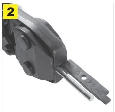
2. Use the Calibration Tool to gauge the jaw gap. Ideally, the jaw gap should be between 0.8 mm and 1.2 mm.
