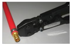
3. Place PEX pinch clamp nub between tool jaws and ratchet the clamp until the PEX Pinch Clamp Tool auto-releases. This action will assure that the PEX pinch clamp is fully engaged.
