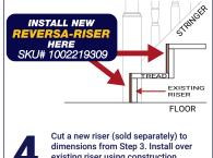
existing riser using construction adhesive and 2" 18-gauge pin nails.
