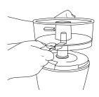
1. Place Juice Bowl (E) on to Motor Unit, lining up the Drive Coupler (M) on the Motor Unit with the hole in the Juice Bowl.
