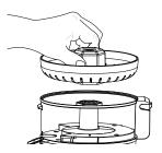
4. Position desired Pulp Filter (J or K) onto Drive Coupler.
