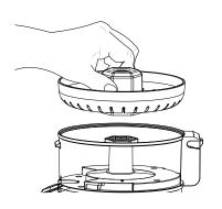
4. Remove the Pulp Filter by pulling straight up to remove it from the Juice Bowl. Dispose of excess pulp.
