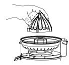
5. Place Reamer (D) onto Drive Coupler and Pulp Filter.
