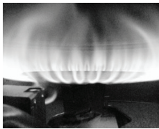
Proper burner and pilot burner pattern.
