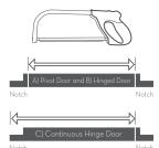
Cut the vinvl to fit your measurement in step 1. A) For Pivot Doors, cut the notches off both ends B) For Hinged Doors, cut the notches off both ends
