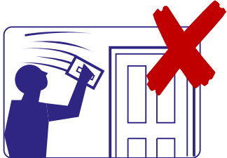
Do not fit any door in a newly plastered room until the air moisture content is down to normal domestic levels
