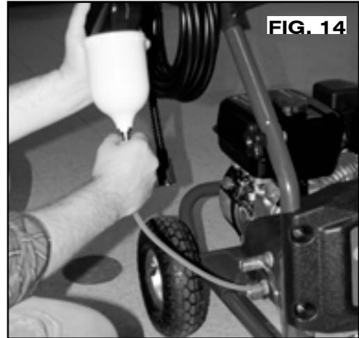
5. Pull engine starter rope slowly several times until antifreeze/ washer fluid comes out of high-pressure hose connection of pump.
