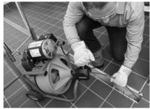
Figure 15 - Operating K-400 with AUTOFEED
