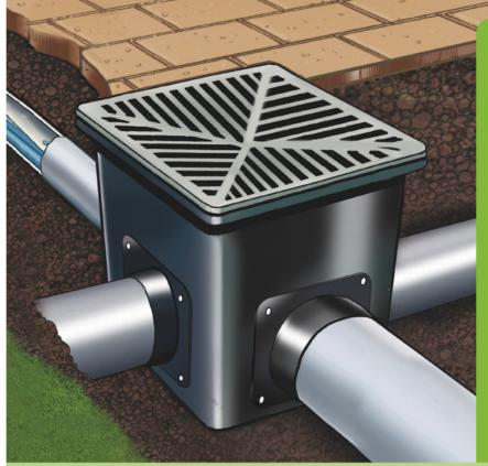
US Trench Drain's PIT BOSS provides an easy, quick and simple method of securing 4" Triple wall pipe to polypropylene catch basins or stormwater pits.
