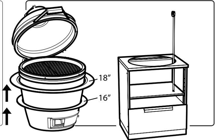
**3** Select the diameter ring according to Kamado size and test from step 2
