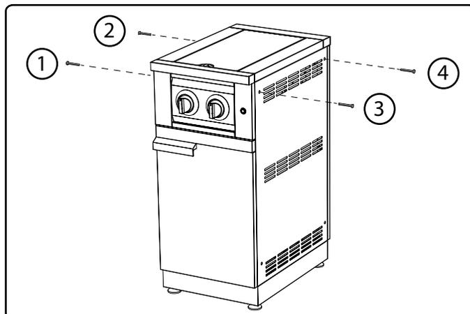
**3** To add an additional cabinet, 60mm bolts need to travel through mounting holes on both cabinets.
