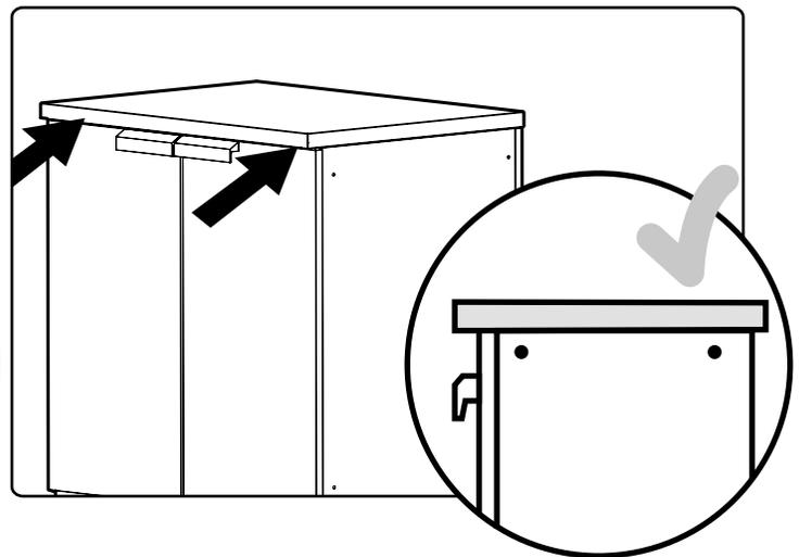
**5** Tighten screws to secure cabinets.
