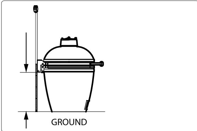
**2** Adjust shelf height to dimension from step 1, test rings for fit, slide up for fit.
