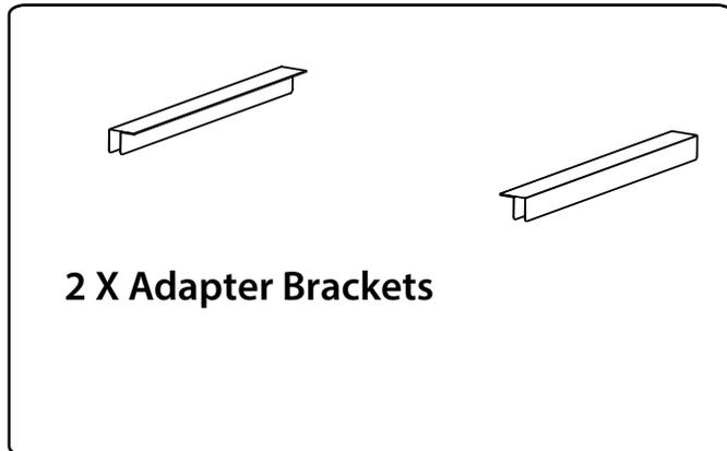
**2** Place BBQ so that the rails touch the Brackets. Lift up edges of BBQ and Dab a little silicone on the rails to hold it in place.
