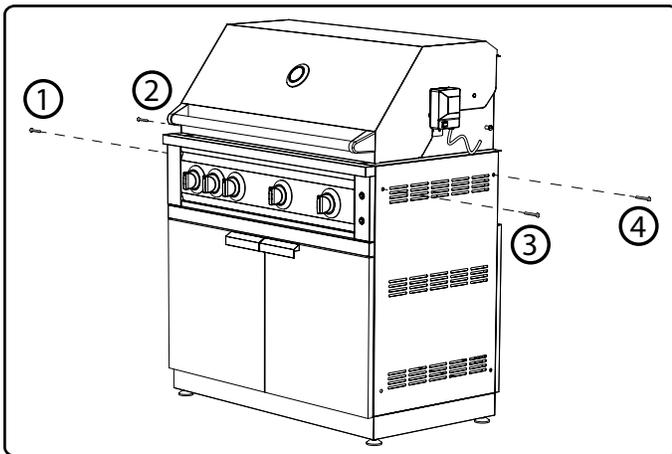
Secure grill to cabinet by inserting four through mounting holes that line up with insert nuts on the side of the grill fire box.
