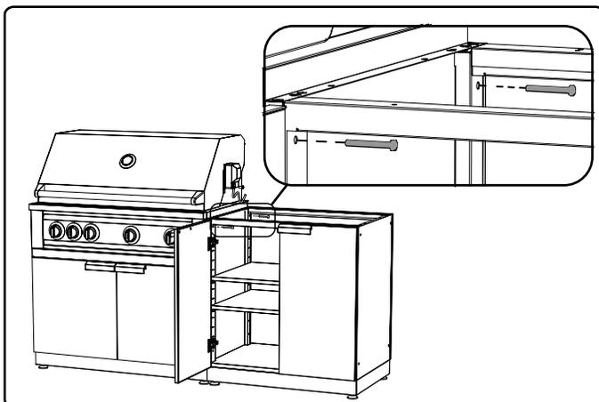
To add an additional cabinet, 45 mm bolts need to travel through mounting holes on both cabinets.
