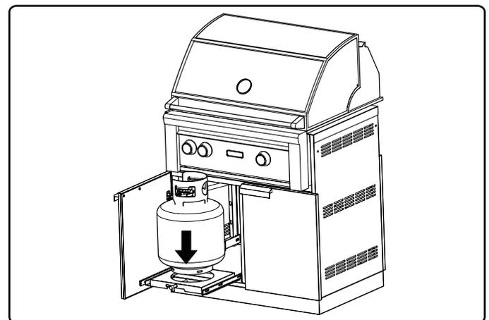
**5** Once tank tray it pushed to the back of the cabinet, lock the tank tray by pushing down on the lock button. Push the release button to unlock.
