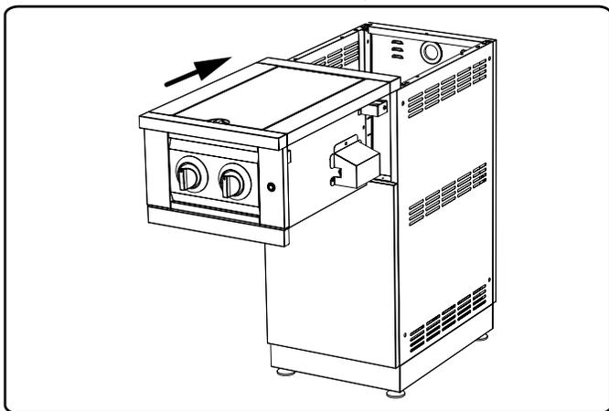
**2** Secure DSB to cabinet by inserting four 50mm bolts through cabinet mounting holes that line up with insert nuts on DSB.
