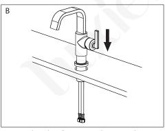
B. Attache the flange and insert the faucet through the mounting hole on the countertop.
