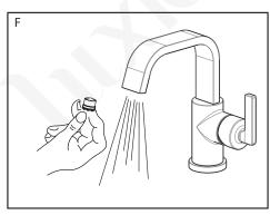
F. Remove the aerator with a small coin or a flat head screwdriver and let the water run for about 1 minute to clear any debris in the plumbing system. Check for leaks at all connections. Reinstall the aerator to complete the installation.
