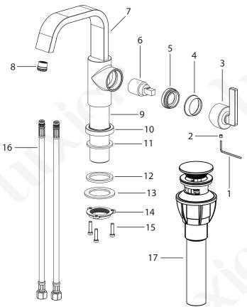
(**Note**: Sediments or mineral buildup will clog the aerator and decrease water flow. It is recommended to clean the aerator regularly to maintain proper water flow.
