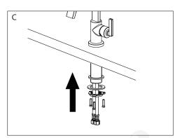
C. Under the sink, slide the washer and metal washer onto the faucet. Secure the faucet with the locking nut and screws to the countertop.
