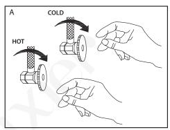
A. Shut off water supply at the valves. Remove the old faucet and clean the mounting surface for installation of the new faucet.
