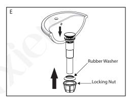
E. Remove rubber washer and locking nut from the drain assembly and slide the drain into the sink. Install the rubber washer first and tighten the locking nut to install the drain.
