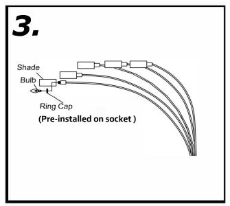
Place the **Shades**, **Ring Caps**, and **Light Bulbs** onto the tips of the **5 Arch Pipe** through the **Light Bulb Socket**.
