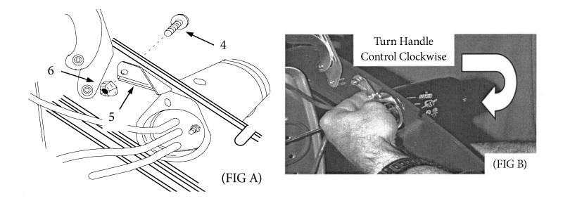
To release Reflector Pan and Heating Element from the vertical Rotisserie position, rotate the Handle Control clockwise slightly to release the pressure from the Rotisserie Lock. Lift Rotisserie Lock up with left forefinger and rotate Handle Control back to horizontal element position. (FIG B)
