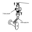
Attach the 7/8" T-valve shutoff to the threaded fill valve on your toilet. Be sure the 7/8" flat washer is in the T-valve before installing. Position the T-valve so that the shuttoff handle is facing the front of the toilet.
