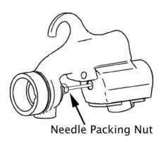
It is a good idea to apply Light Machine Oil or Vaseline to the Needle Shaft where it passes through the Needle Packing Nut and work it in and out by pulling the Trigger back and forth. This will lubricate the Needle Packing #12.
