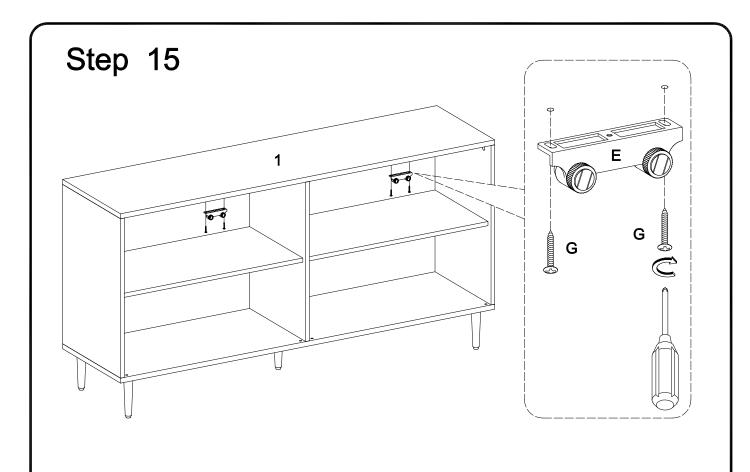
Secure door stopper (E) to top panel (1) with screw (G).
