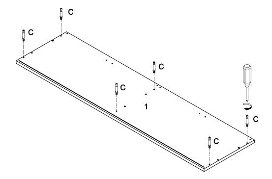
Secure cam bolt (C) to top panel (1).
