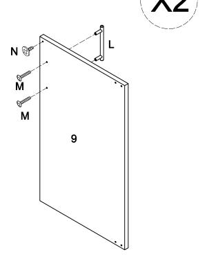
Secure handle (L) to door (9,10) with handle bolt (M), and secure bolt (N) to door (9,10). Repeat this step.
