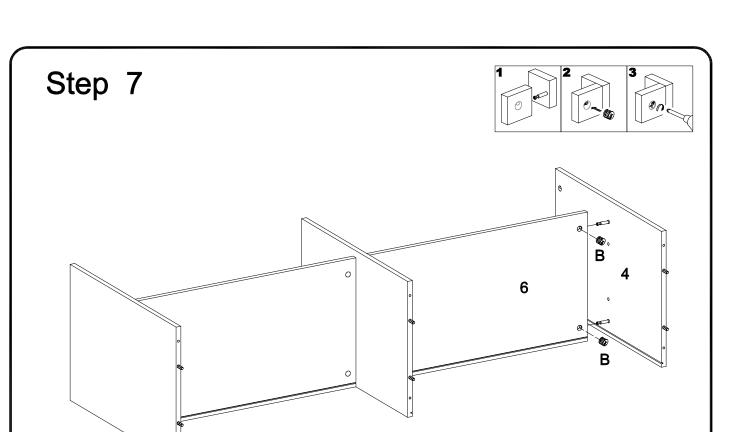
Insert side panel (4) into shelf (6), then insert and secure cam lock (B) to shelf (6) to lock it.
