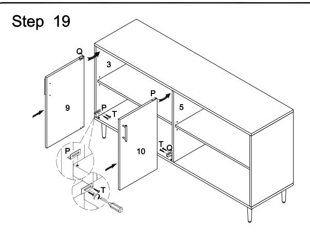
Insert door hinge (P,Q) into panel hole as per diagram. Slide door (9,10) onto door hinge as shown in diagram and secure it with screw (T).
