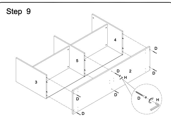
Use wrench (H) to secure bottom panel (2) to side panel (3,4,5) with bolt (D).
