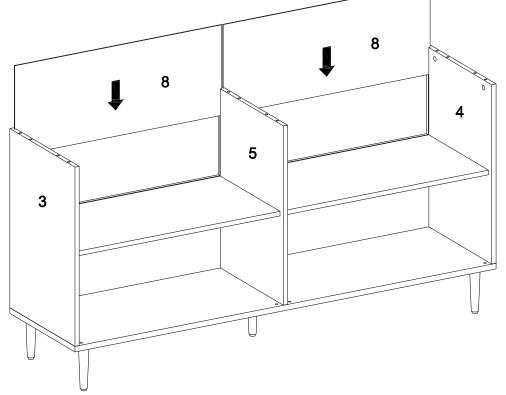
Slide back panels (8) into grooves as per diagram.
