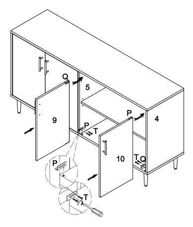
Insert door hinge (P,Q) into panel hole as per diagram.
