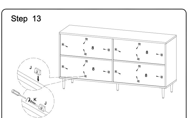
Secure plastic wedge (J) to back panel (8) with screw (K).
