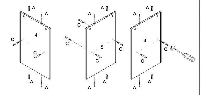
Insert wooden dowel (A) and secure cam bolt (C) to side panel (3,4,5).
