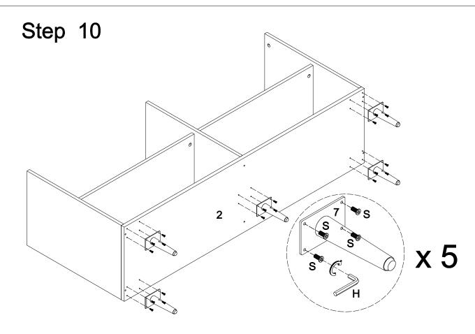
Use wrench (H) to secure leg (7) to bottom panel (2) with bolt (S). Repeat this step five times.
