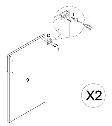
Secure door hinge (P) to door (10) and door hinge (Q) to door (9) with screw (T). Repeat this step.
