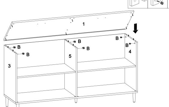
Insert top panel (1) into side panel (3,4,5), then insert and secure cam lock (B) to side panel (3,4,5) to lock it.
