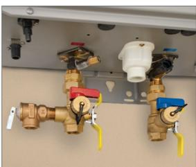
Seal the threaded connections with an approved Teflon® tape. Pipe dope is not recommended. When tightening the fittings, use a wrench for support. **DO NOT** overtighten as damage to the fittings can occur.
