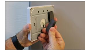
Remote will have a magnet on the back for easy mounting directly to the unit cabinet. If mounting on the cabinet, skip to step 8; if mounting on a more accessible wall location, continue reading.
