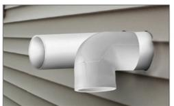
From the outside, locate and mark a center line for the exhaust vent location. Mark a center line 5-1/2" to the right of the center of the exhaust for the air intake vent. Ensure that the exhaust vent location is at least 12" below or from a window or door. Check all clearances as listed in the "Venting" section of the "Installation Instructions" in the Use Care Manual. **DO NOT** locate the intake and exhaust more than 24" apart.
