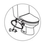
11. Connect the hose from step 6 to the bidet water connection underneath the handle of the HD-4000.
