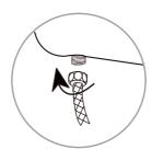
3. Disconnect the water hose from underneath the toilet tank.
