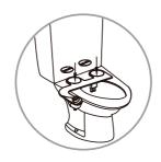
8. Place the circular mounting brackets into the bidet attachment.
