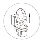
1. Remove the existing toilet seat by locating the bolts and nuts, typically under a plastic cover, and removing them first.
