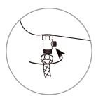
5. Attach the water supply hose that comes from the water shut off to the bottom of the T-Valve.
