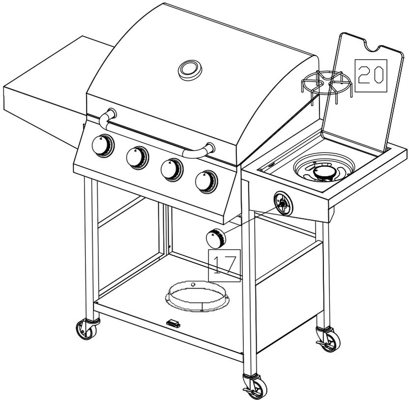
10. Decorated knob (17) is assembled to side burner's front plate. Grate (20) is putted on side burner shelf, with 3 longer legs into the holes.
