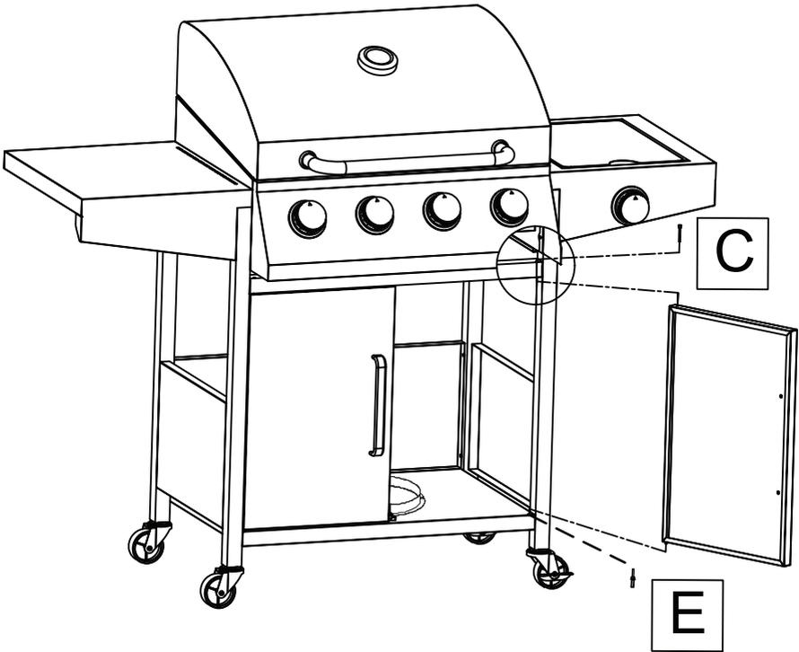
12. Doors are assembled to frames' front legs with top and bottom pins (C&E).
