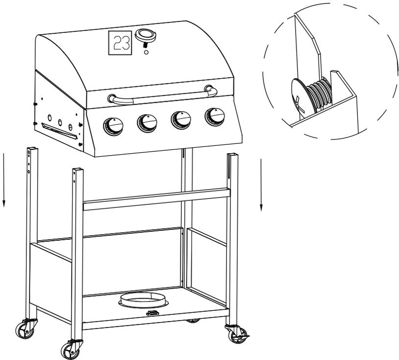
5. The body (1) is slid into the frame legs with 8 pcs pre-assembled M5 screws (See detailed pic.). Tight screws after body slid into position.
