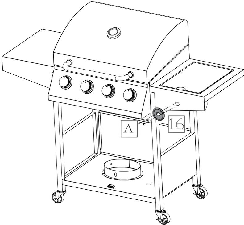
8. Side burner rotary switch base (16), side burner front plate and side burner valve (inside shelf front plate) are assembled together with 2pcs M4 countersunk screws (A).
