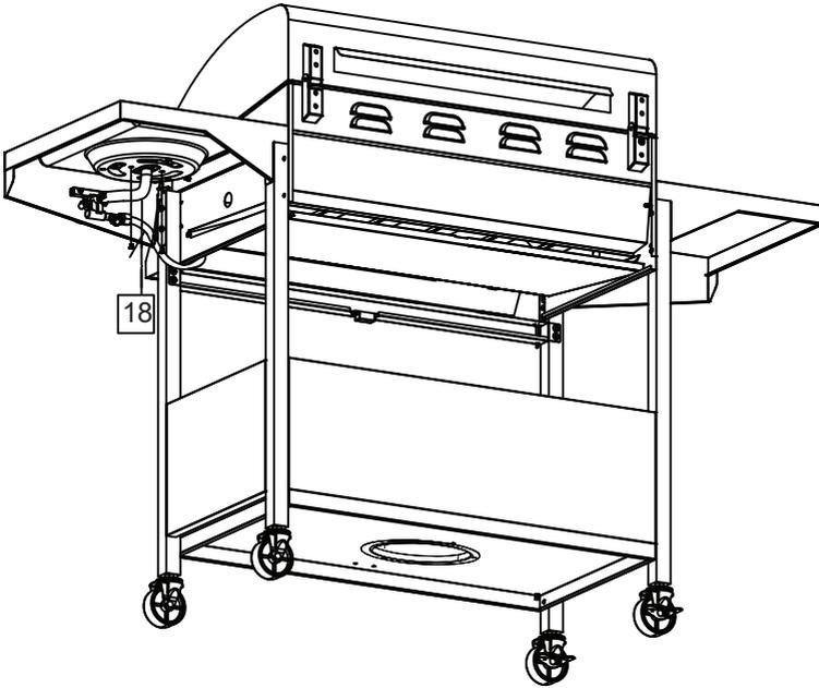
9-1. Side burner (18) is assembled into the side burner shelf with 2 pcs M4 screws (A). Insert the tube to valve connector.
