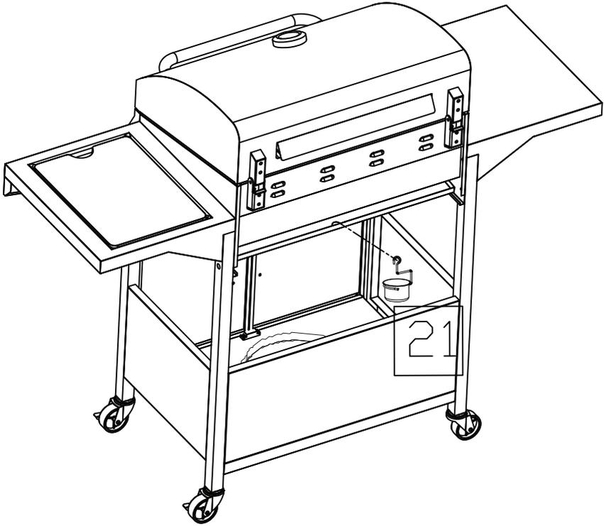
14. Oil cup (21) is assembled to the oil pan.
