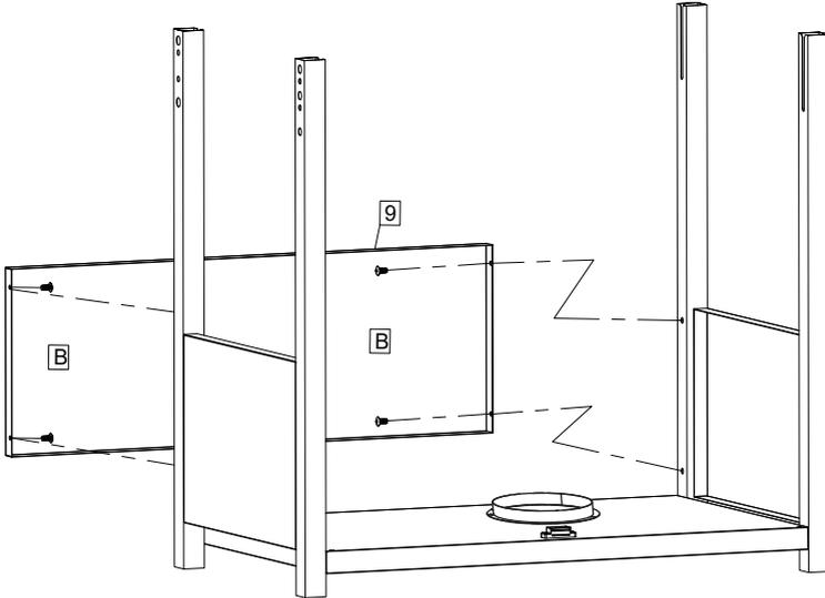
2. Assemble the back shelf (9) to the frames with 4 pcs M5 screws (B).
