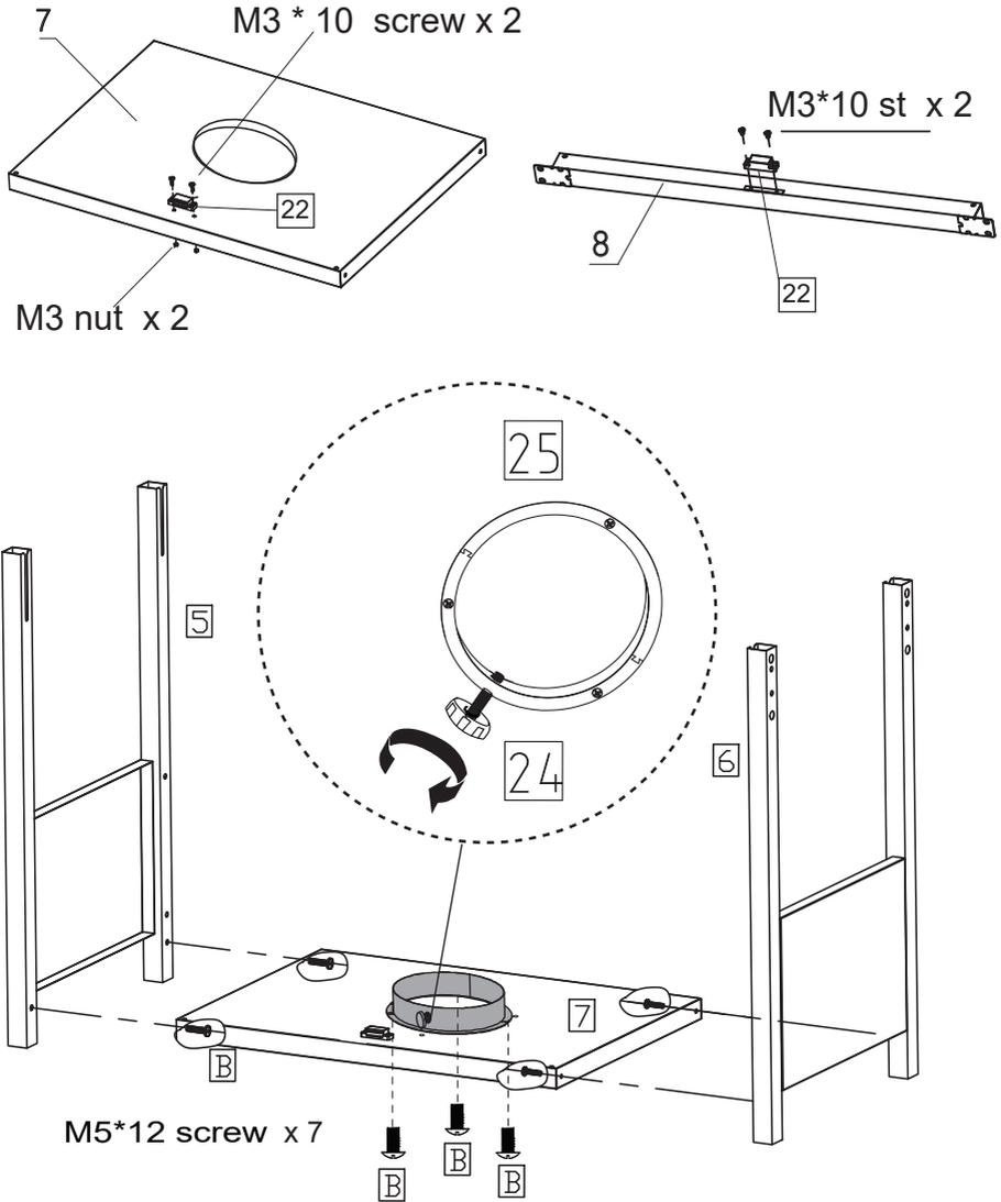
1. Assemble the LH and RH frame (5&6) to bottom shelf (7)
