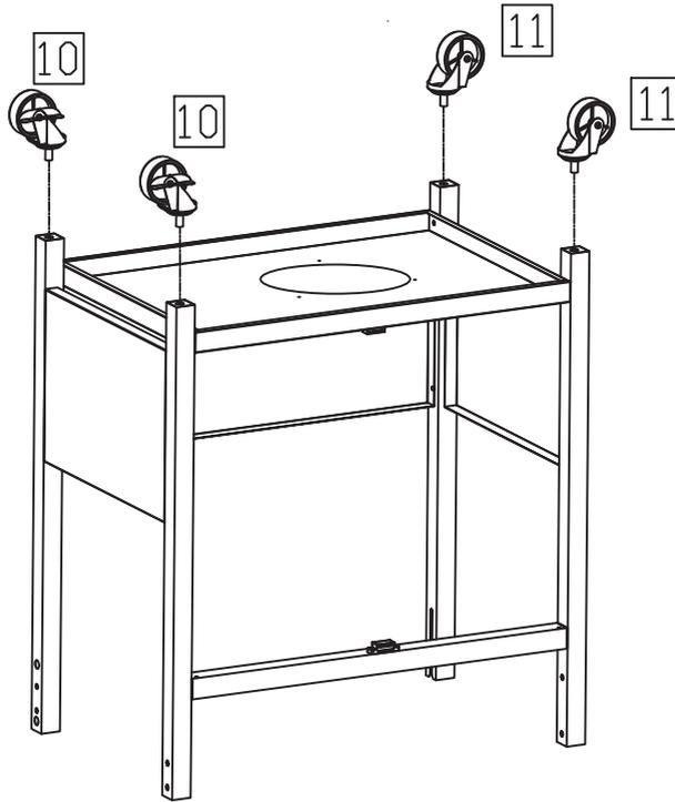
4. Assemble the 4pcs wheels (10&11) to the end of frame legs.
