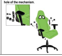
With the seat positioned as shown, assemble the armrests (C) to the seat frame on their respective sides using screws (I), O' rings (M) and washers (N).
