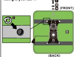
Attach the covers (K) to the brackets on their respective sides using screws (L) and cover the holes with (O). Then place the seat over the base, making sure the tip of the gas lift enters into the
