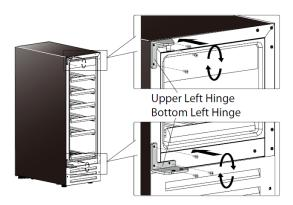
6. Rotate the door  $180^{\circ}$  so that the top is now the bottom, and install it by attaching the support rod with screws.
