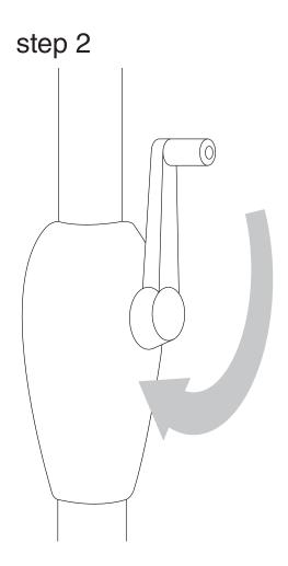
1. Turn the crank handle clockwise until the umbrella is fully opened.
