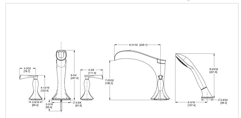
Ø1 Min to Ø1-1/2 Max. Deck Hole Openings
