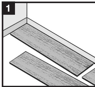
2. Installation should start in a corner (left hand) and proceed from the wall with the tongue facing the wall. Allow a minimum gap of 1/4 in (6 mm) for product expansion, which should be covered by molding (**Figure 2**). Set 1/4" spacers to create the required expansion space.
