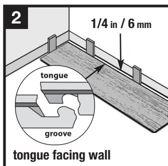
3. When laying the first row in a straight line interlock the short ends by inserting the tongue into the grooves at an angle of approx. 10 to 20 degrees (**Figure 3**). Install each sequential plank on the short end and be sure to line up evenly. Use a soft faced hammer to tap down on top of the planks on the short seam to ensure a tight fit (**Figure 7**). This is very important for a good installation.
