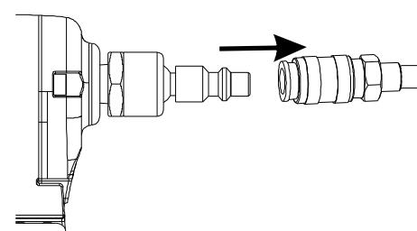
2. Turn the tool so the air inlet is facing up. Place 2-3 drops of pneumatic fastening tool oil into air inlet. Do not use detergent oils, oil additives, or air-tool oils as these lubricants will cause accelerated wear to the seals and bumpers in the tool, resulting in poor tool performance and frequent tool maintenance.
