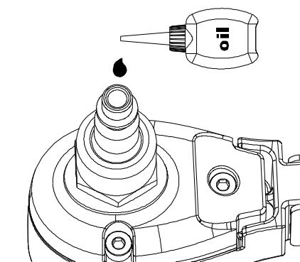
3. After adding oil, connect the tool to the air source, run tool briefly. Wipe off any excess oil from the cap exhaust.
