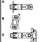
Some locksets are supplied with 4-way latch which can fit either mortise-in or drive-in.
