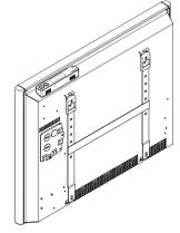
THE BOTTOM OF THIS UNIT MUST BE INSTALLED AT LEAST 4 INCHES (10.2 CM) FROM THE FLOOR.
