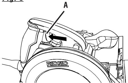
A - Switch trigger (commutateur, interruptor)
