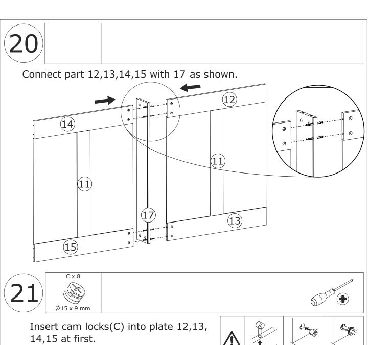
Turn cam locks clockwise to tighten.
