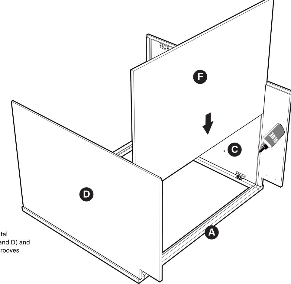
Run a bead of wood glue in the lower horizontal grooves in the Frame (A) and End Panels (C and D) and slide the Fixed Shelf (F) completely into the grooves.
