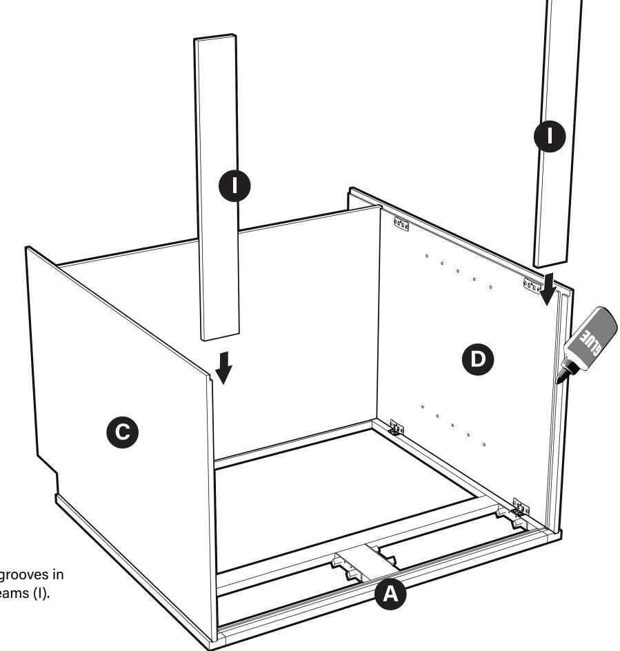
Run a bead of wood glue into upper horizontal grooves in the End Panels (C and D) and insert the (2) I-beams (I).
