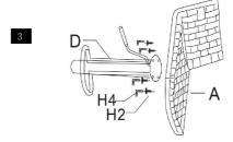
Step 3 Align the column (D) onto middle of the frame as pictured. Use allen key "H4" to lock the 4 screws "H2".
