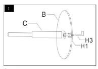
Step 1 Align the gas lift (C) onto the base as pictured. Use allen key "H3" to lock the 3 screws "H1".
