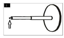
Step 2 Remove the black cap on the top of the gas lift.
