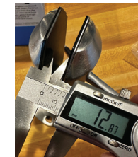
Lever Spigot with shim insert. Shim the opening is approximately 12.9mm.
