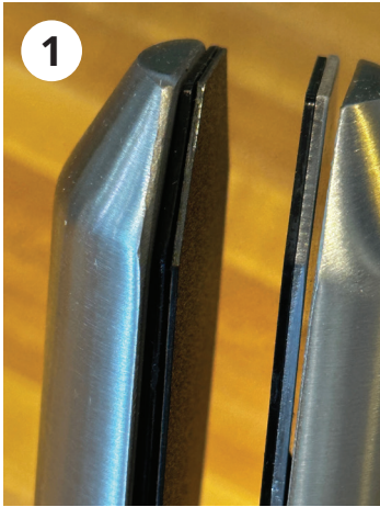
1 Determine if there is a shim in the Lever Spigot insert.
