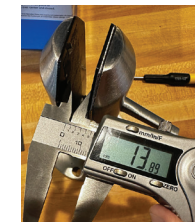
Lever Spigot without shim insert. Shim the opening is approximately 13.9mm.
