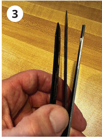
3 Remove the shim from the Lever Spigot insert and set aside.
