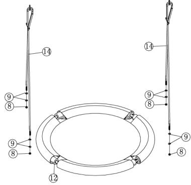
Attach the other end of the Swing Rope(#14) into the Carabiner(#7) secured to Top Bar(#A).
