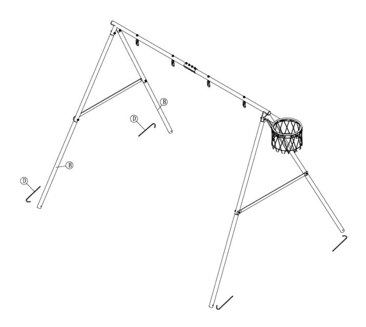
Slide the Tube(#12) into the sleeve of Flying Saucer(#13), and then connect the 4 tubes together.
