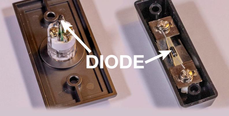
If a diode is not installed on a push button, install one diode on the "front" push button.
