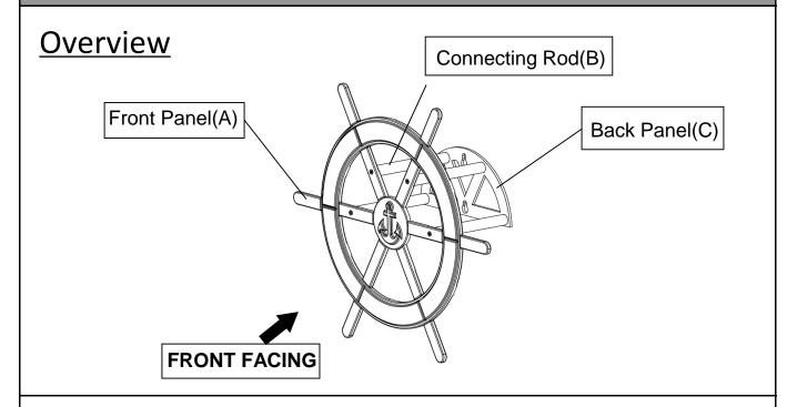
This product has multiple parts and may require up to some 30 minutes to assemble. To give you an overview of the hose holder parts, the above picture is to help you put the various parts into perspective.
