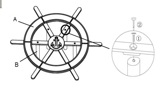
Attach Front Panel(A) to Connecting Rod (B) using Bolts(1) with Screwdriver(2). Do not over tighten.
