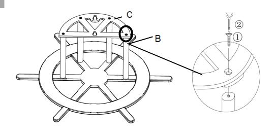
Turn the hose holder over, make Front Panel(A) facedown as pictured above. Attach Back Panel(C) to Connecting Rod (B) using Bolts(1) with Screwdriver(2).
