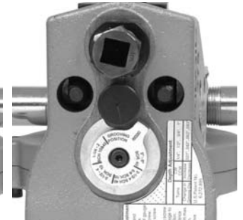
Figure 15B – Gauge In Grooving Position
