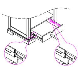
Pull the right clip upward and left clip downward at the same time, then draw the drawer box out.
