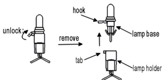
Fig. 1 Unlock and remove the burned out lamp
