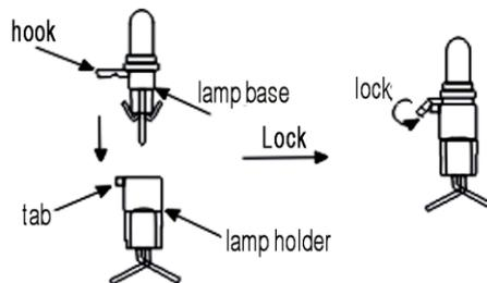
Fig. 2 Replace with the spare lamp
