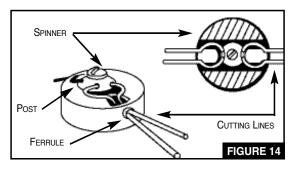
WARNING: Use only .080 diameter monofilament cord 12 3/4" long. Use of thicker lines, lines made of substitute materials, or lines greater than 12 3/4" long MAY RESULT IN PERMANENT DAMAGE TO YOUR MOTOR AND/OR INJURY.
