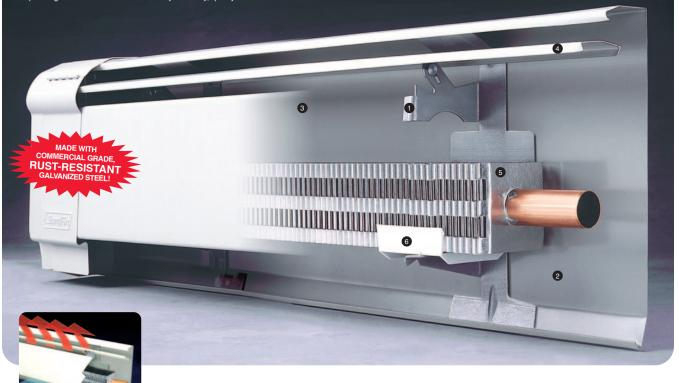
Wall streakage eliminated. Top panel and damper form a shield to keep dust from settling into baseboard interior, and to deflect heated air away from the wall, into the room. Back panel has no holes or slits to leak air behind the back of the baseboard causing wall streakage.
