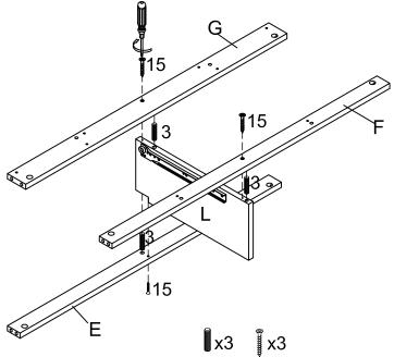
Step 3. Attach assembled parts E, F, G & L to Side Panel C with Wood Dowels & Cam Locks as shown. Attach Back Rail D to Side Panel C with Wood Dowels & Cam Locks as shown.
