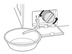
**5** Clean the pump filter and opening.
