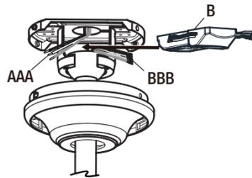
Receiver (B) correctly positioned in the mounting bracket.
