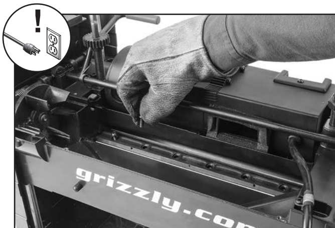
Figure 22. Example of removing screws securing knife to cutterhead.
