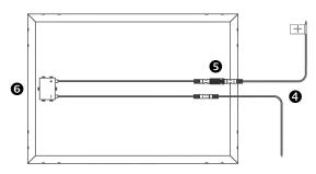
Connect the bare wire end of the positive cable 4 to the "SOLAR +" input of the charge controller 1. Connect the negative bare end 1 to the "SOLAR -" input. Now, you can mount the Comet-40 to an indoor wall or within a NEMA-3R rated enclosure.
