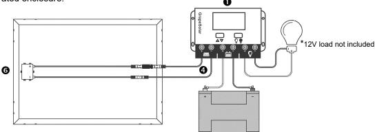
Remove the panel covering. In good sunlight, the charge controller's • "BAT %" should increase to 100%. Once the battery is fully charged and the controller is set to "LOAD ON," the system will provide power through the load control output or through the two USB ports. If an inverter is added to the system, it must be connected to the battery bank, and not to the charge controller.
