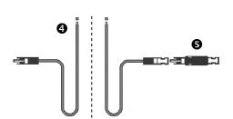
Connect the MC4 ends of the halved cable
