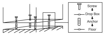
Mount the safe by running screws from inside of the safe and securing to anchors; ensure the parcel drop box mounted securely.
