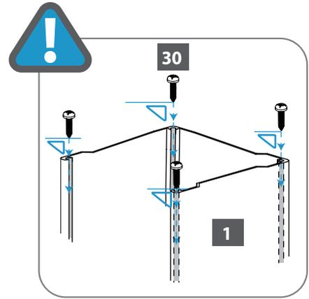
Leave support frames (2) about 10" over lower end of corner profiles (1) until step 4 ( Securing the gazebo to the ground)
