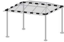
**NOTE:** The Long Rail (5) and the Short Rail (7) have a preassembled connecting part to be inserted into Long Rail (6) and Short Rail (8).
