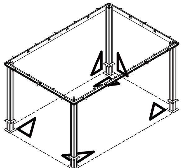
**IMPORTANT:** After this step you should place the gazebo frame in its desired location. Make sure all corners are squared at 90 degrees.
