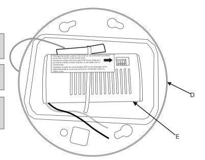
The receiver (E) is pre-installed into the mounting plate (D).
