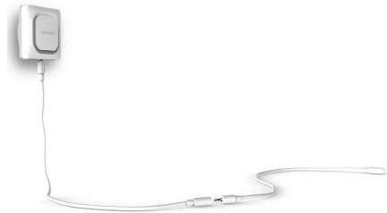
Fig. 1. Plugging in additional cable sensors.
